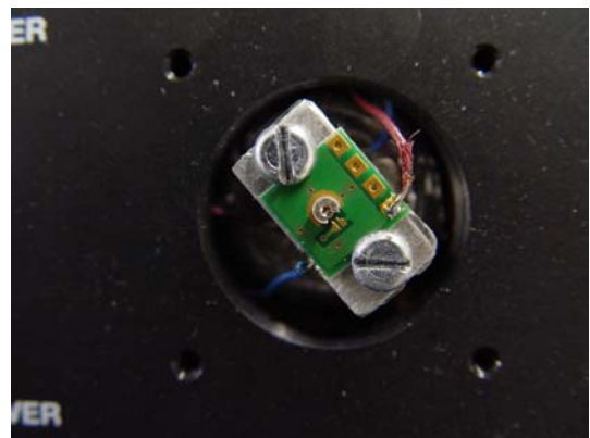
Figure 8: Laser module placed in the diode mount
