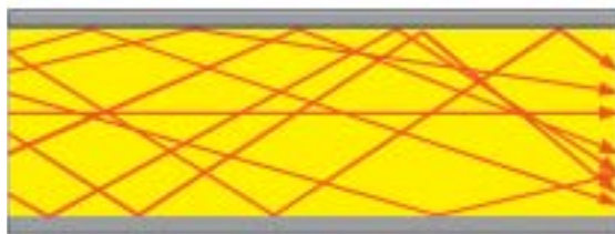
1 The principle of step index wave-guides
