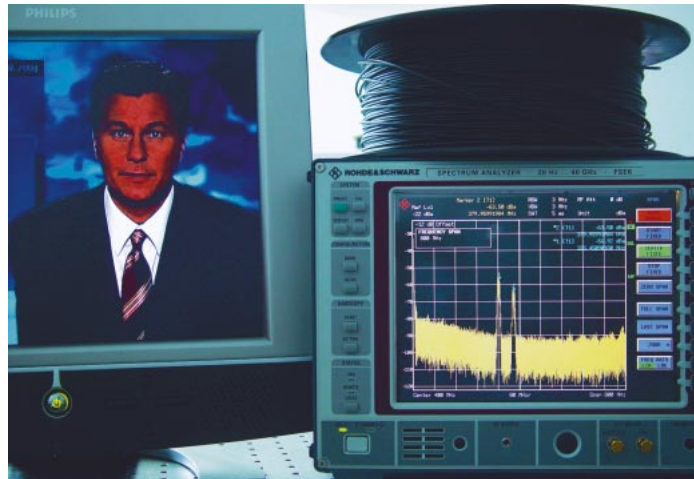
Figure 2: Transmission of TV signals with 50 m of polymer optical fiber (POF)
