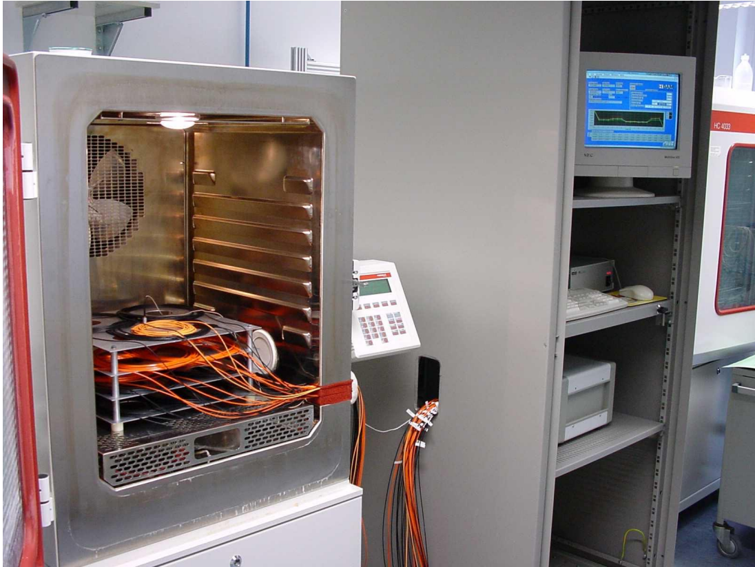
Fig. 1: Climatic chamber with PC-controlled multiplexer
