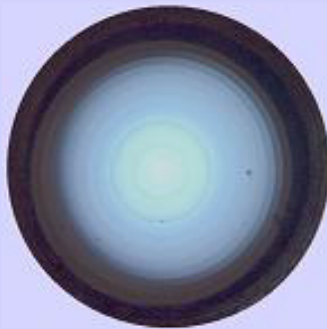
1 mm POF PMMA-GI 1000 Mbit · 100m
