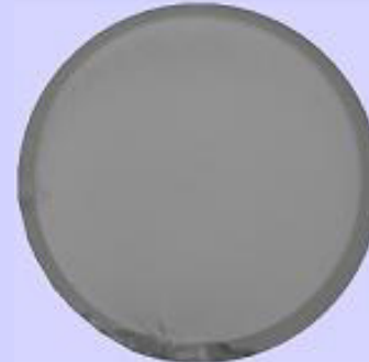
1 mm POF PMMA-GI 1000 Mbit · 100m
